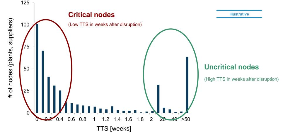
If the TTS of a particular node is smaller than the expected time to bring the node back to full functionality (TTR), the disruption will expose the supply chain to financial and operational problems.
